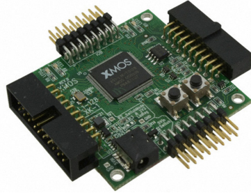
Fig. 10 XMOS XK-1A board
