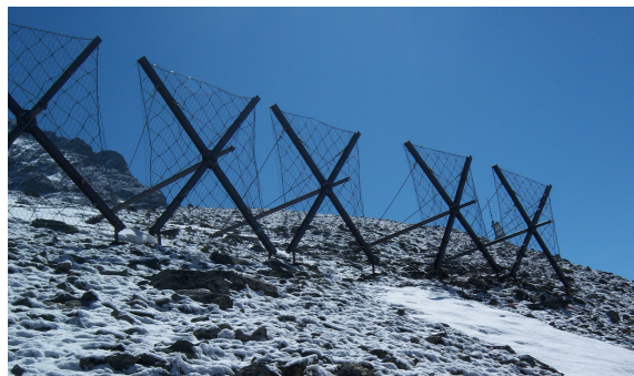
Figure 3: Arrays of snow umbrellas at the experimental site of Localité-La-Tour, Valsavarenche, photo De Biagi.
