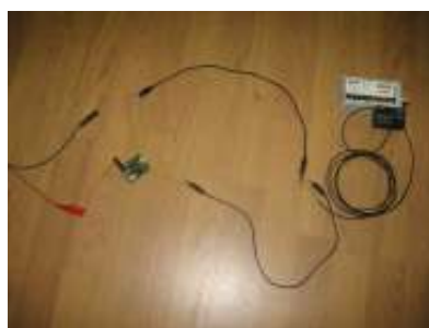
Figure 7.9. Smart grid node during the massive stress test connected to commercial pulse generator which will be connected to the gas meter in a real application.
