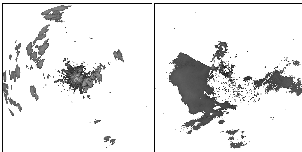
Figure 2.8. Example of grayscale .png images acquired by the radar installed in Turin in clear sky days without clutter filter (on the left) and by the radar installed in Palermo during a heavy rainfall event (on the right).
