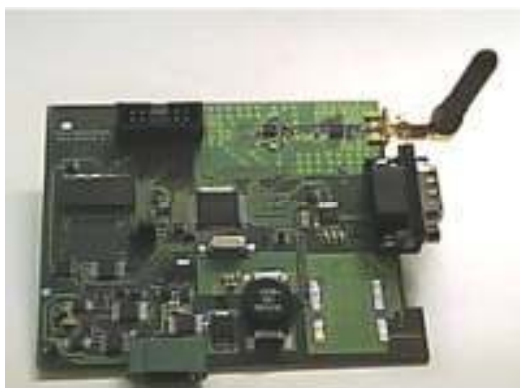
Figure 7.1. Sensor board used in the WSN designed as anti-theft alarm system for PV Panel.
