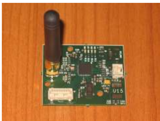
Figure 7.4. Realized electronic board for gas smart grid nodes.
