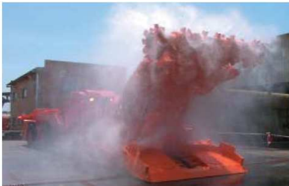
Fig. 6. Roadheader fitted with a de-dusting system used as a possible winning means in critical formations
