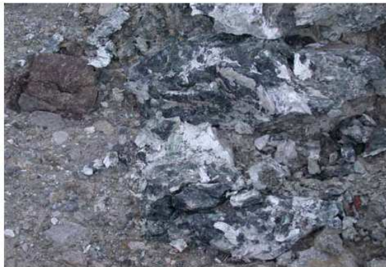
Fig. 3. Asbestos elements in the fractures of heaped muck intended for reuse
