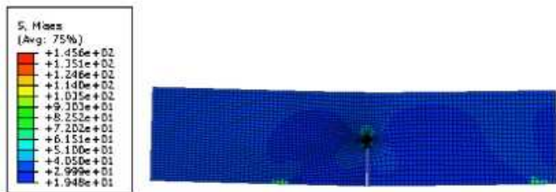
Fig 7.32: Stress distribution inside the model for 80V and crack length of 10 and 20 mm
