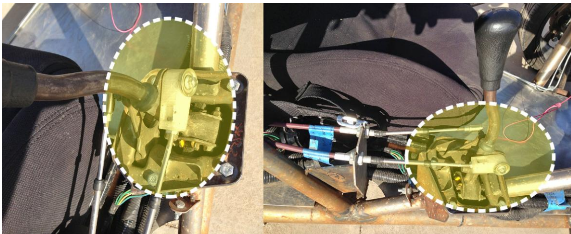
Figure 27: Connection part to fix a gear lever, produced with a 3D printer in the Local Motors Microfactory
