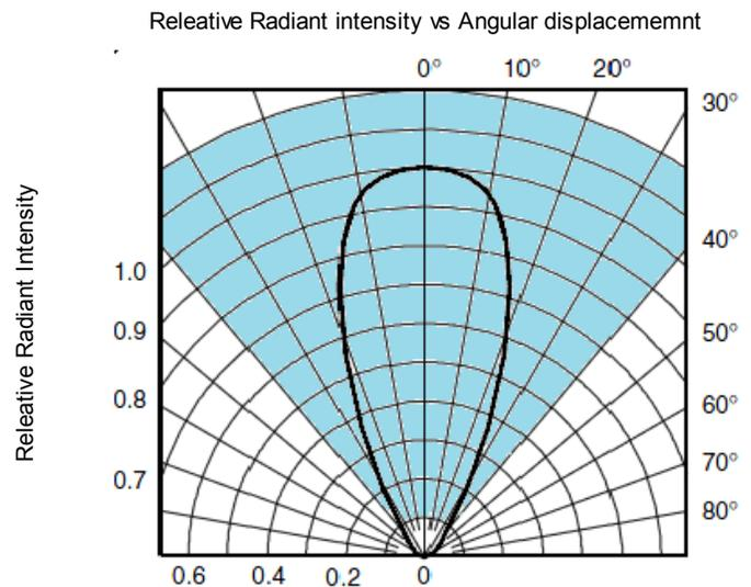
Fig.3 Relative Intensity vs Angular Displacement, courtesy Vishay [5]
