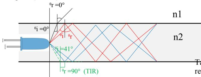
Fig. 4 Optical light guidance in the Fiber
