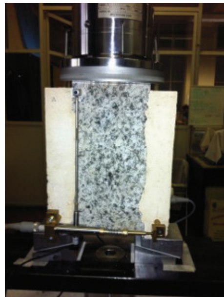
Fig. 10 Composite specimen stone-repair mortar.
