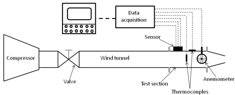
Figure 4: Schematic diagram of the experimental facility (see Ref. [18]).
