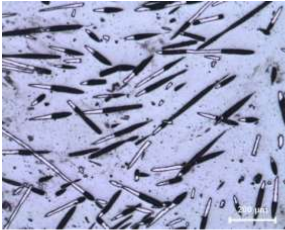
Figure 27: 10 % short fiber reinforced \beta -SiAlON composites hot pressed at 1650 °C [43]
