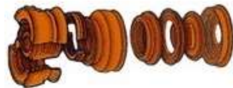
Figure 16: Exploded view of the core major module of the CFM56-7 engines [26]
