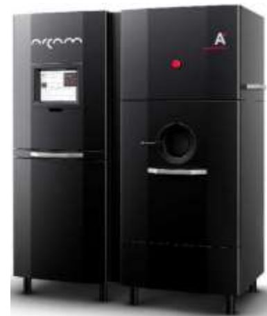
Figure 72: Arcam A2 machine [119]
