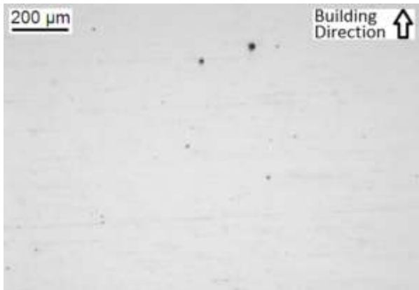
Figure 86: Micrograph showing the typical porosity in as-built sample from powder Ti-48Al-2Cr-8Nb
