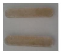
Figure 7.5: Cured samples obtained by swelling according to method 1(up) and 2 (down)
