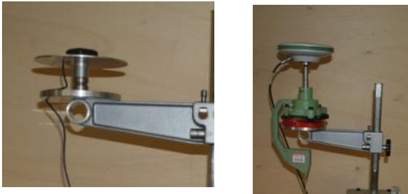
Figure 13. Antenna support: patch (left) and geodetic (right)
