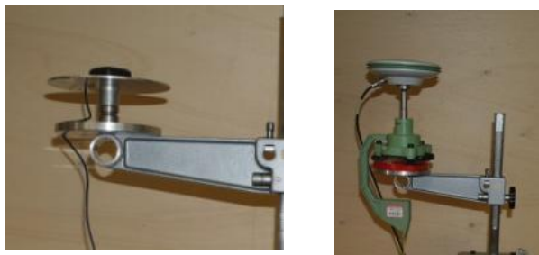
Figure 13. Antenna support: patch (left) and geodetic (right)
