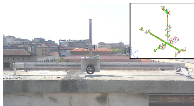
Figure 12. Micrometric slide for controlled deformations
