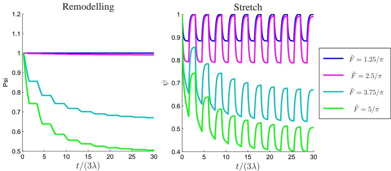
Figure 3: Cycle of compressions, when a constant external force  $\tilde{F}_M$  is periodically applied and then removed: reorganization (on the left) and stretch (on the right). The simulations are performed setting  $\tilde{\tau} = 0.625$  and  $\tilde{\mu} = 1.6$ . The compression and release times are both equal to  $\tilde{t}_c = \tilde{t}_r = 3/2$ . From top to bottom the applied force increases.
