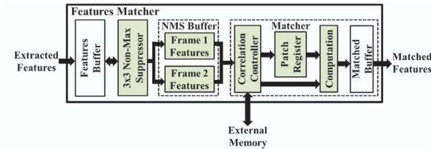
Fig. 4: *Features Matcher* internal architecture
