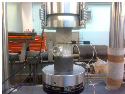
Figure 13: Experimental set up of the compression test on the concrete specimen.
