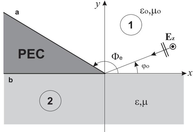
Figure 1: Perfect electric conductor (PEC) wedge aperture angle  $(\pi - \Phi_e)$  lying on a dielectric half-space and illuminated by a E-polarized plane wave at normal incidence with direction  $\varphi_o$ .
