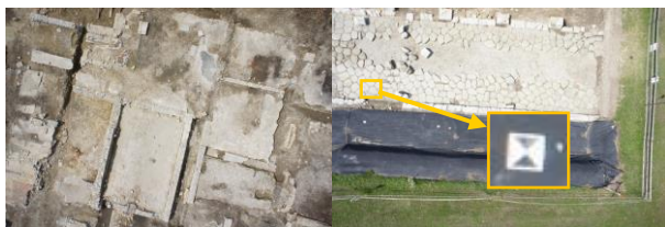
Figure 8 Two acquired images in the area of Via Gemina: high flight (left) and low flight with a zoom on a target (right).
