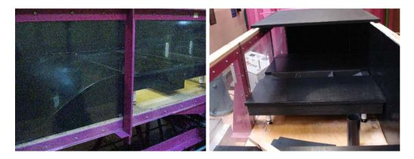
Figure 2.3. Pictures of the convergent ramp, supports and flat panels.
