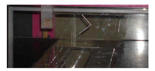
Figure 2.8. Detail of the hot wire probe holder. Flow is from left to right.
