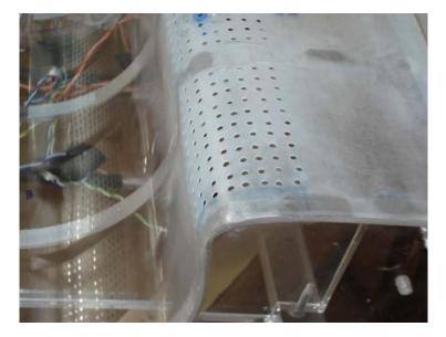
Figure 2.6. Detail of the porous surface on the downstream cavity edge, in region B.
