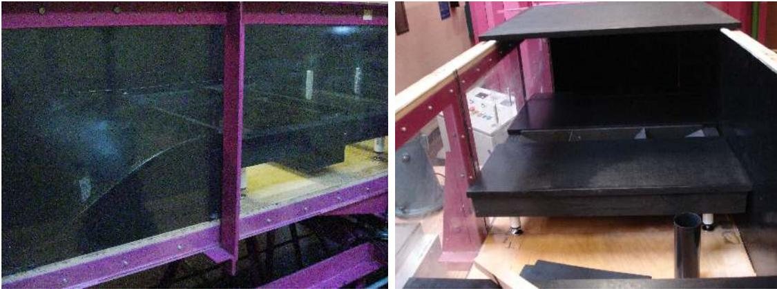
Figure 2.3. Pictures of the convergent ramp, supports and flat panels.
