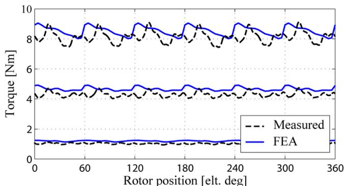
Fig. 14. Prototype 3C: torque waveforms on the MTPA.
