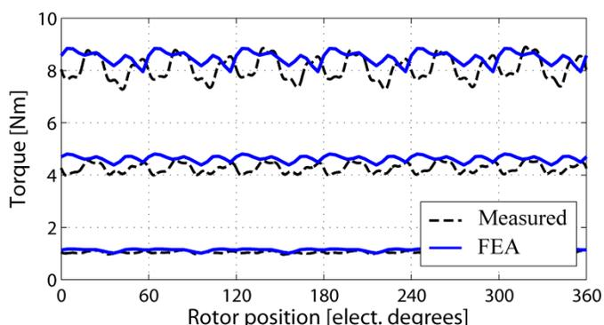
Fig. 18. Prototype I2U: torque waveforms on the MTPA.
