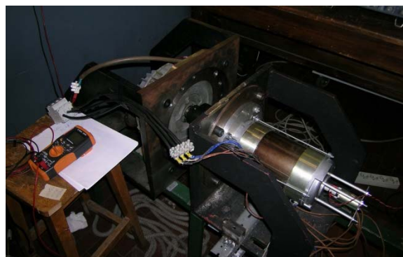
Figure 13. LSSyR motor prototype loaded by the DC machine.
