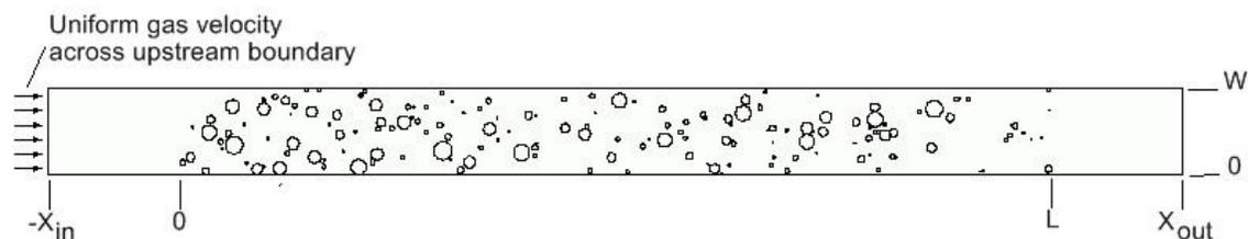
**Figure 1. Typical 2-Dimensional Flow Domain for CFD Simulation of Fibrous Filter Media**
