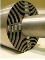
Figure 6. Rotor lamination of the motor under test
