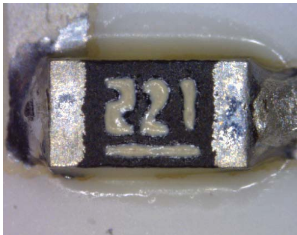
Fig. 6. Microscope picture of a resistor soldered with lead solder paste on the inkjet printed microstrip.
