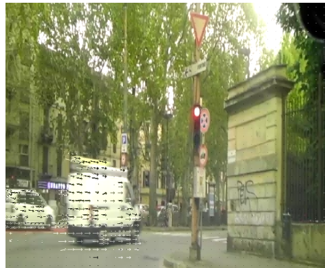
Fig. 2. Crossing vehicles at a traffic light stop. Several high-magnitude motion vectors are present even if the car is not moving.
