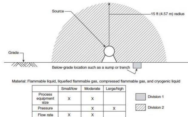
Fig. 1. Leakage of compressed flammable gas located outdoor
