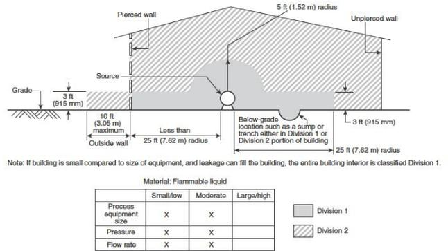
Fig. 4. Leakage of flammable liquid located indoor, ventilation not adequate
