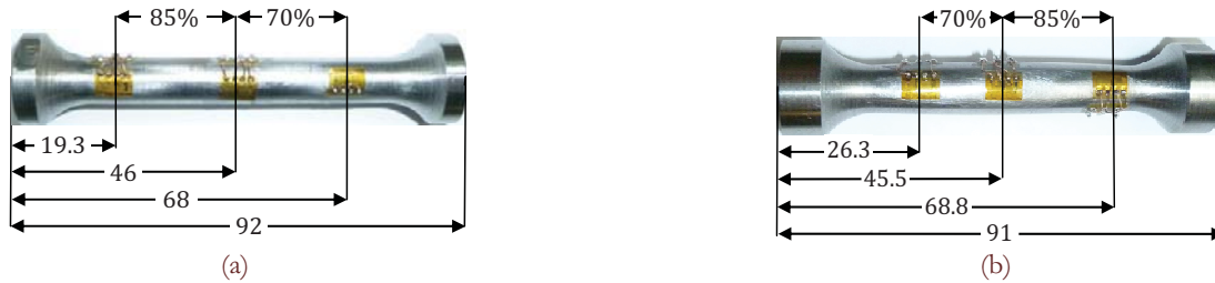
Figure 6: Specimens after application of strain gage rosettes: (a) dog-bone shaped specimen; (b) Gaussian specimen.
