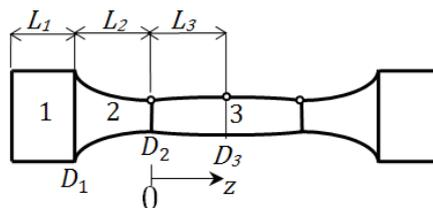
Figure 1: Gaussian specimen.
