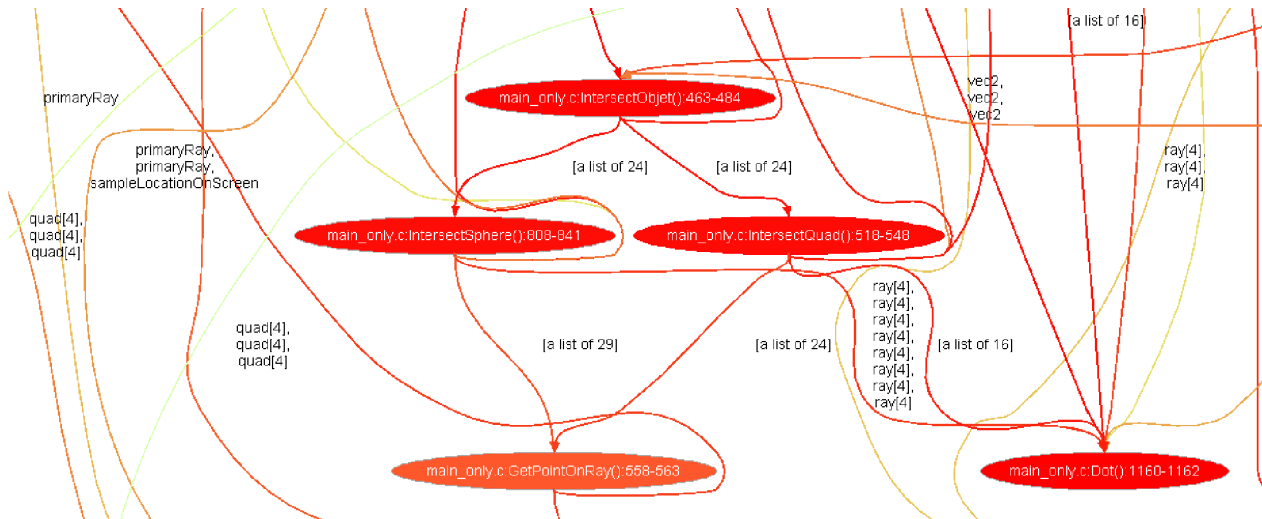
Figure 11. Data dependency traces around the intersectObject function of the ray tracer.
