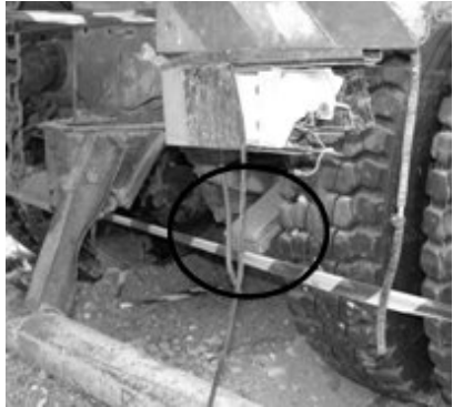
the couple of collapsed leaf springs
