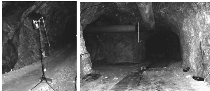
Figure 1, 2: Measurement of the air flow in underground by means of anemometer at node "N20"
