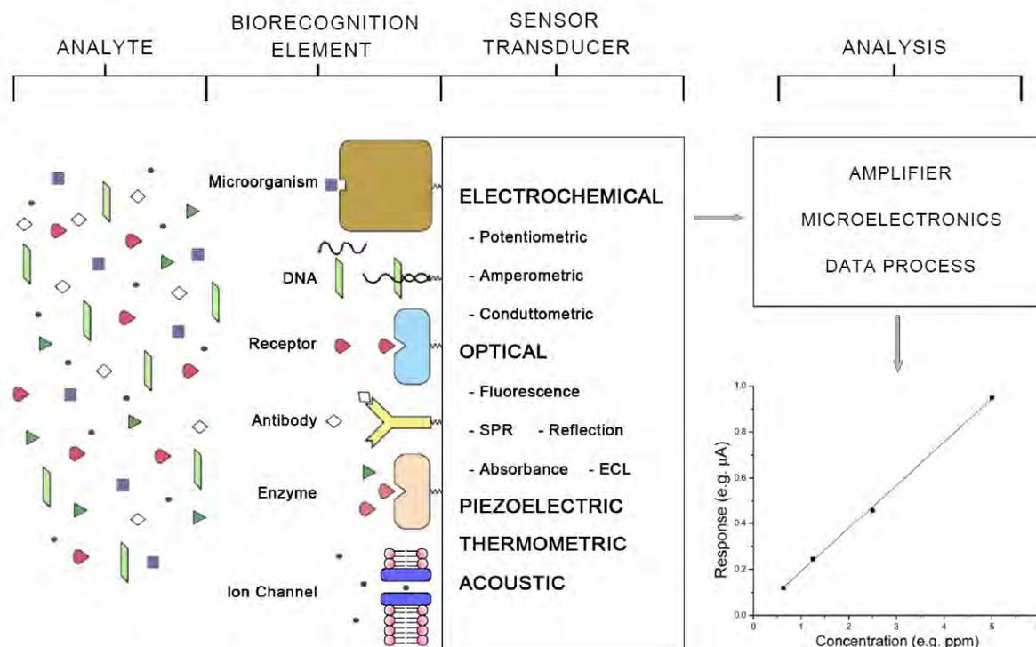
Figure 2.1: General scheme of a biosensor.
