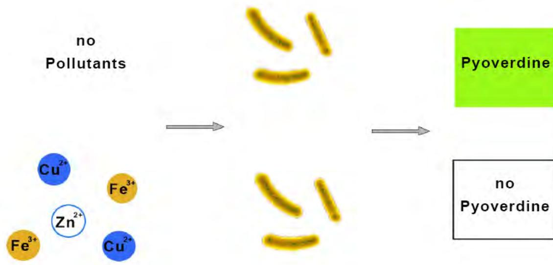
Figure 3.8: Scheme of a biosensor for environmental monitoring based on *Pseudomonas* response to metals.
