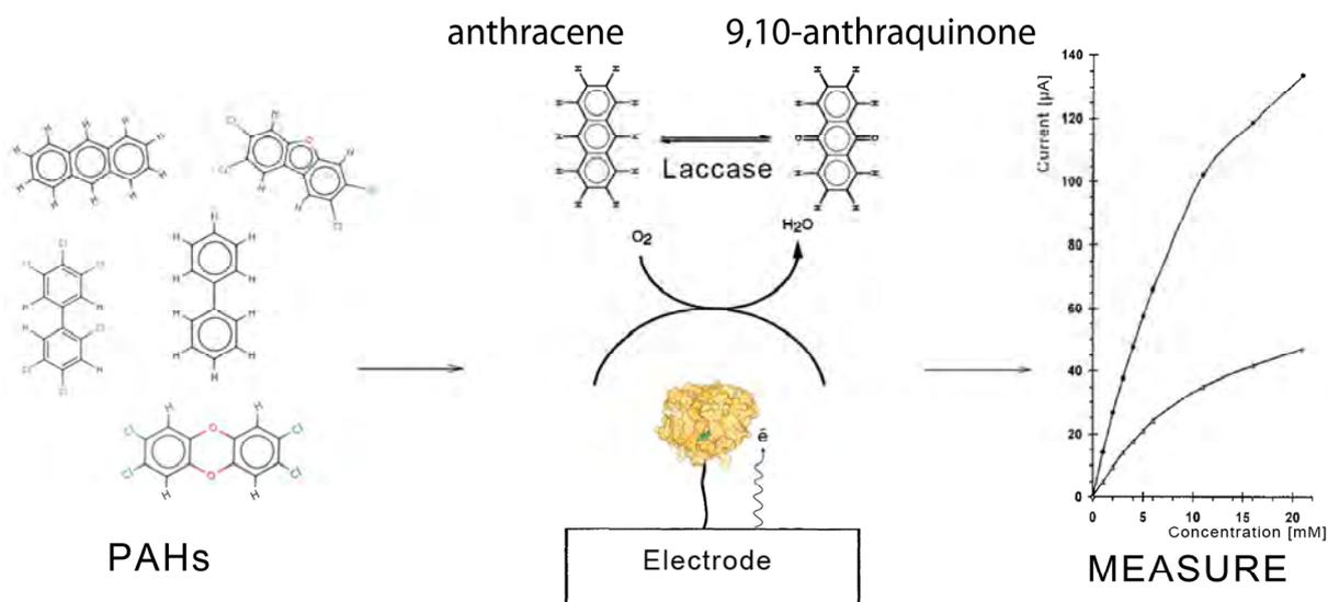
Figure 3.10: General scheme of a biosensor for PAHs detection based on a modified laccase enzyme.
