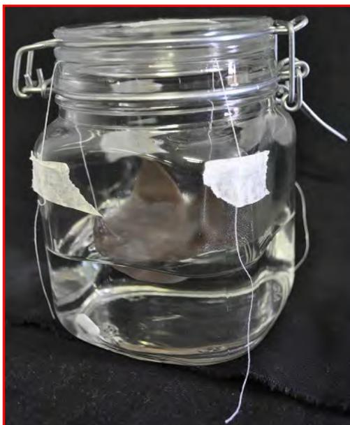
Figure 4.3: Image of the PVA release test.
