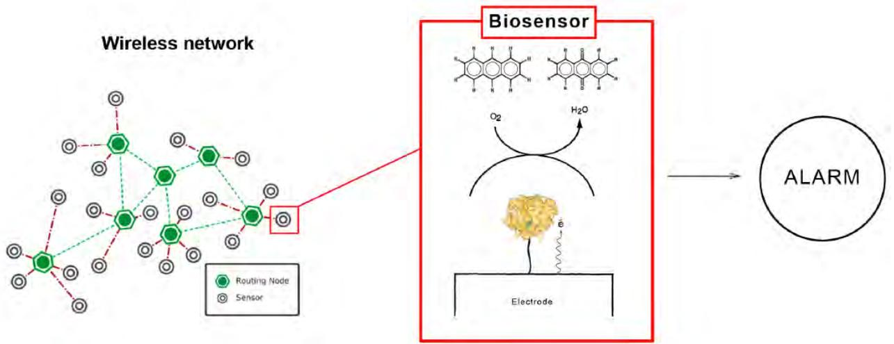
Figure 3.1: General scheme of a BEWS based on an enzyme biosensor implemented into a wireless sensor network.
