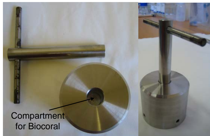
Figure 3.13 : Mortar and pestles. Mortar is made of stainless steel, autoclavable and liquid nitrogen resistant.
