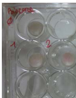
Figure 3.4 : Biocorals placed in wells of a 24 well-plate. Growth medium will fill the well completely covering the Biocoral.
