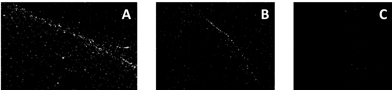
Fig. 5.7 SHG images of collagen (in white) spiked in fibrin gel with at concentrations of 0.05 mg/ml (A) and of 0.01 mg/ml (B) and without collagen (C).
