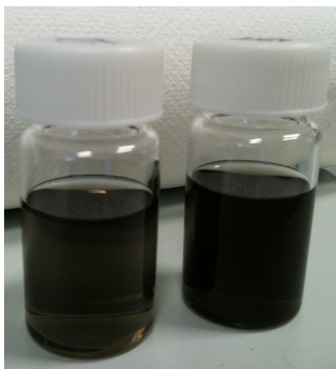
Figure 3. Graphene dispersion in DMF
