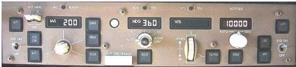
Figure 25. Boeing B-777 autopilot modes panel
