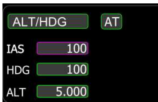
Figure 101. Example of Guidance Data on Main Display
