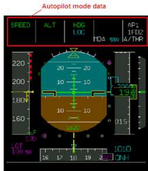
Figure 26. Autopilot mode data on Airbus A-380 PFD
