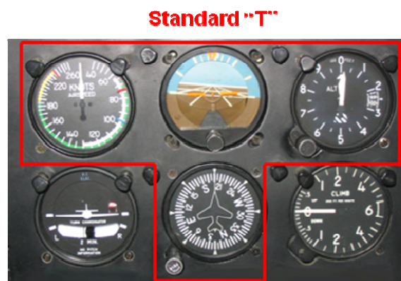
Figure 105. Example of Standard “T” Layout in a Traditional Cockpit
