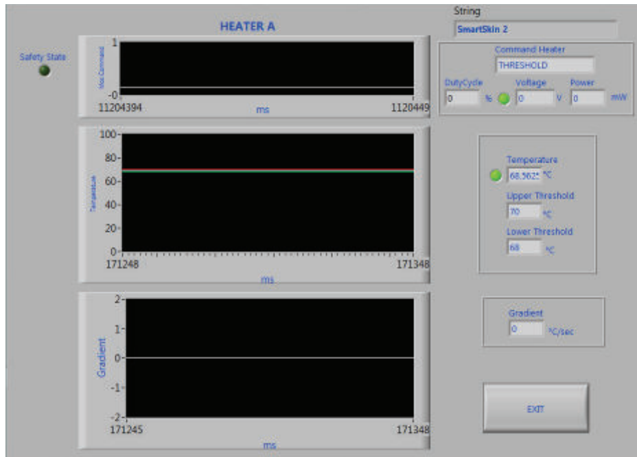
Figure 4.13: Case 1 - Heater A on smart skin 2 (dissipated power is 0 because the temperature is above the minimum threshold).
