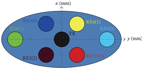
FIGURE 5: Sample fiber bundle for MC analysis. RX1–RX4 fibers are centered in  $x, y = \pm 1$  mm and retracted by 0.5 mm, 2 mm, 0 mm, and 1 mm on the  $z$ -axis, respectively; RX5–RX6 are centered at  $x = 0$  mm and  $y = \pm 3$  mm and retracted by 0 mm and 1 mm.
