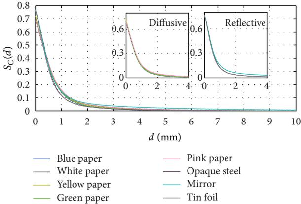
FIGURE 12: Evaluation of the  $S_C(d)$  curves for the different targets. Left inset zooms on the close-range portion for diffusive paper targets, and right inset zooms on more reflective targets (steel, mirror, and tin foil).
