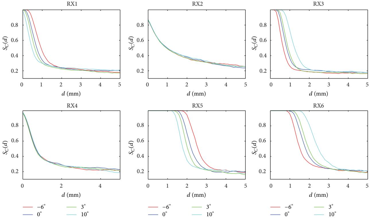
FIGURE 8:  $S_C(d)$  functions for each RX fiber for a horizontal target rotation of  $-6^\circ$ ,  $0^\circ$ ,  $3^\circ$ , and  $10^\circ$ . RX2 and RX4 fibers, the most retracted from TX along z-axis, appear to be rotation insensitive, as they are more shadowed.
