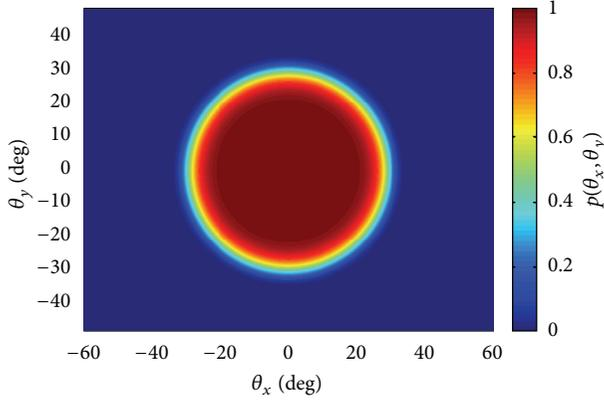
FIGURE 4: Ray acceptance probability for a super Gaussian emission matching the field profile of a standard step-index POF. Parameters:  $G = 3$ ,  $\varphi_C = 28.03^\circ$ ,  $\sigma = \varphi_C^{2G}$ , and  $\alpha_x = \alpha_y = 0^\circ$ .
