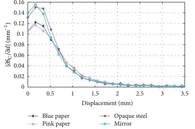
FIGURE 13: Sensitivity of the  $S_C(d)$  curves with displacement.
