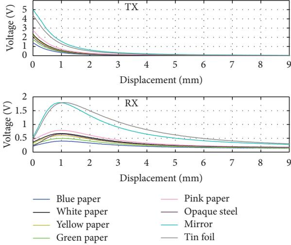
FIGURE 11: Experimental  $V_{TX,C}$  and  $V_{RX}$  curves as a function of target displacement, for 8 different target profiles. An offset  $V_{OFF} = 1.91$  V has been subtracted from all TX voltages to compensate for directivity of the POF coupler.
