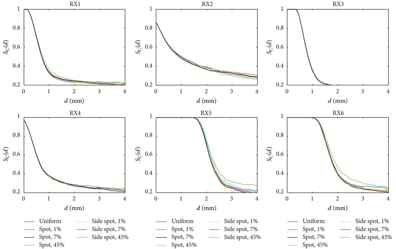
FIGURE 9:  $S_C(d)$  functions for all RX fibers in presence of a spatially nonuniform target reflectivity; the chart reports result for a circular spot with radius 2 mm and with reflectivity variation of 1%, 7%, and 45% from the target nominal reflectivity, either facing the TX fiber (spot) or centered 1 mm aside along  $x$ -axis (side spot).
