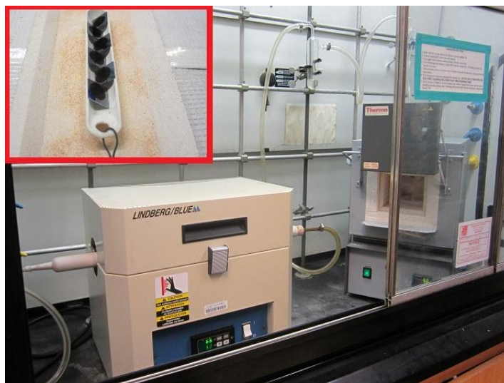
Figure 2-7 Box oven and tube furnace utilized for the polymerization and carbonization steps, respectively. The inset shows some CPS composite chips at the final stage.
