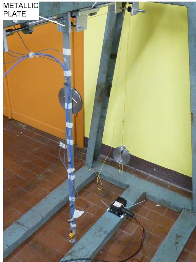
Figure 10.3. Complete structure. At the top, the plate added to the system to enforce the clamp is highlighted. The travelling mass and the counterweight are observable on the left and on the right, respectively.
