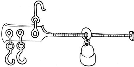
A balance or a steelyard to weigh the bucket.
