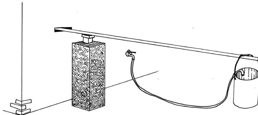
A testing machine capable of applying the load at a uniform rate with water or sand has to be prepared.
