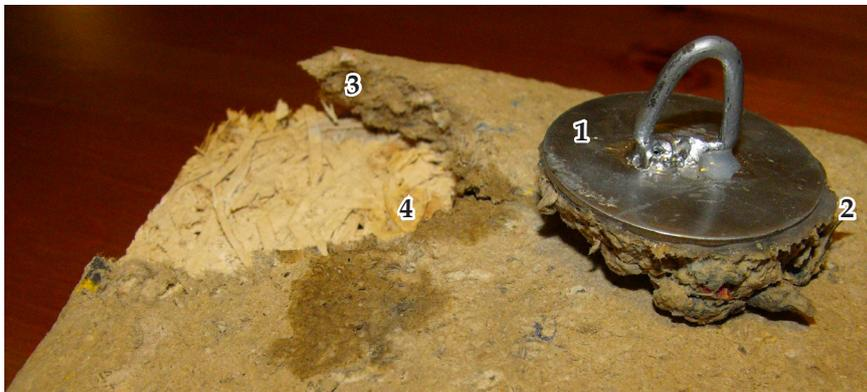
**Type of fracture a - Fracture of adhesion - Fracture between the mortar and the support. The test value is equal to the force of adhesion**
