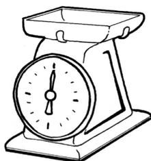
An instrument – accurate as much as possible – to weigh the total mass of the specimen.
