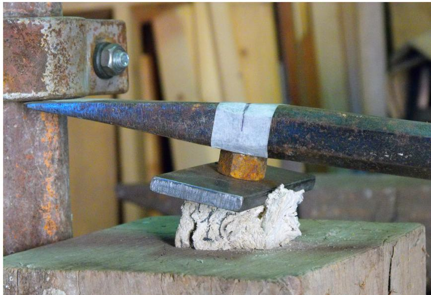
Calculate the strength as the maximum load carried by the specimen  $\cdot 10$  plus the weight of the lever.
