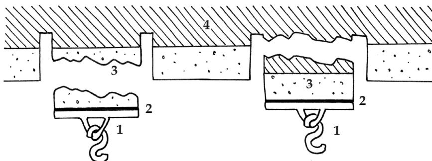
**Type of fracture b - Fracture of cohesion - Fracture in the mortar itself. The adhesion strength is greater than the test value**
