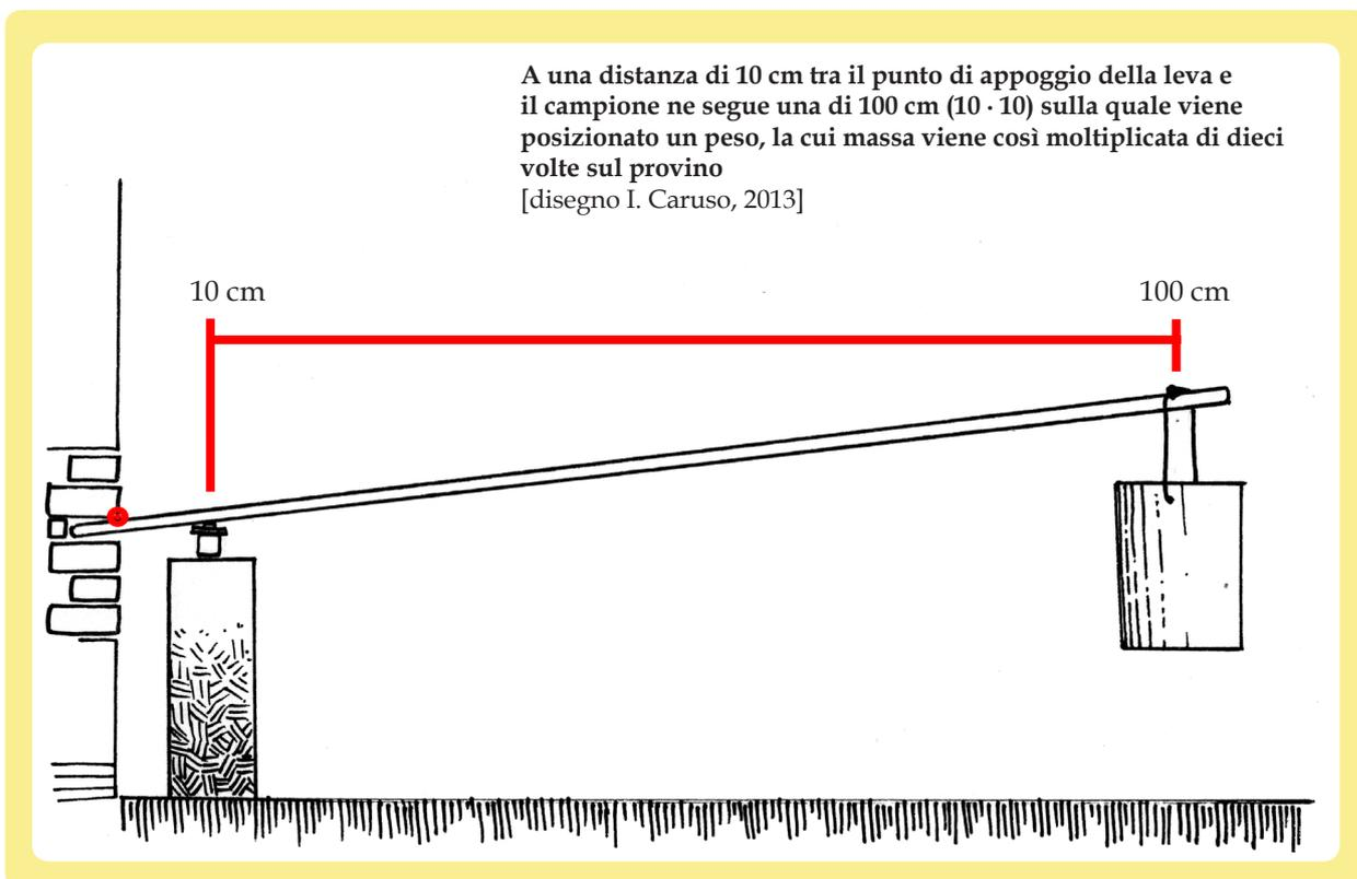
The compressive strength of the mortar is determined on the two parts resulting from the flexural strength test, if not damaged, applying a compressive load on specimens to crush
