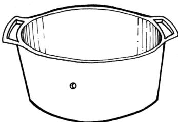
Bucket or basin, with a minimum depth of 20 mm and a flat-bottom big enough to immerse a specimen and equipped with a device for maintaining a constant level of water (for example a hole just above the water level by maintain)
