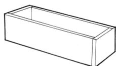
Metal moulds (or any other smooth material), whose dimensions are 40 x 160 mm and depth 40 mm.
