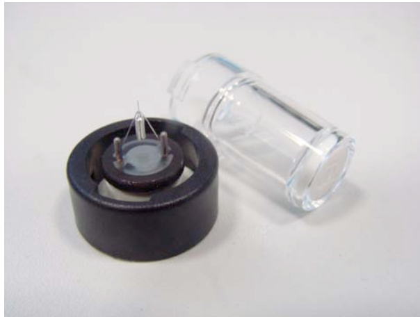
Figure 8.1. FEI Quanta™ 3D LMIS Ga + ions source
