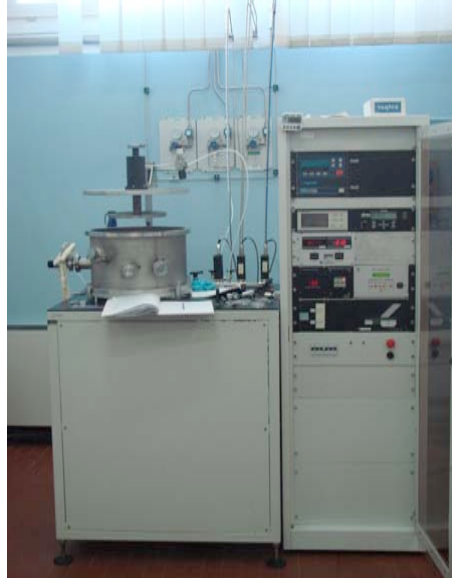
Figure C.2. Picture of the Reactive Ion Etching system, at INRIM. This system is equipped with \text{CF}_4 , \text{CHF}_3 , \text{O}_2 , and Ar gases.
