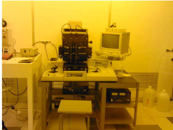
Figure C.5. Picture of the Quintel-Neutronix mask aligner for optical lithography, in the “Thin Film” ISO5 clean room Laboratory.
