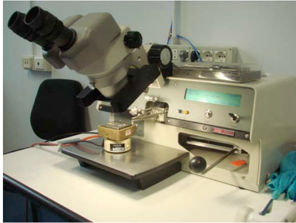
Figure C.7. Picture of the wedge bonder used to realize the micro-contacts from lithographic pads and macroscopical stripes.
