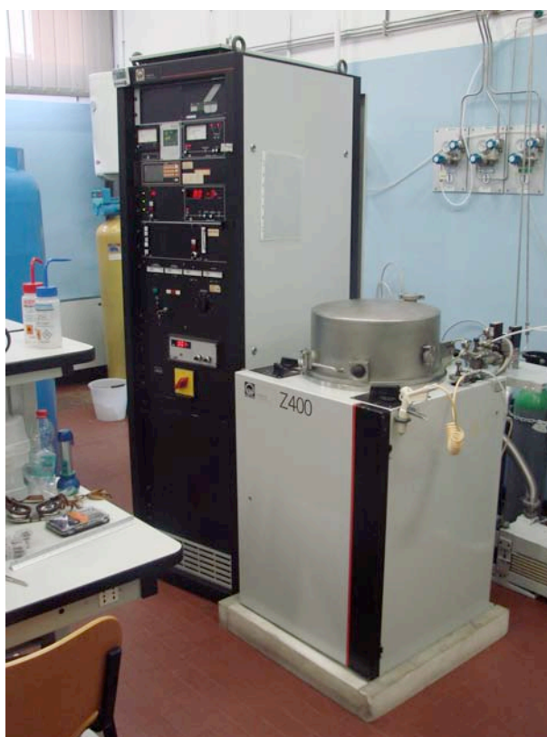
Figure C.1. Picture of the Leybold high vacuum RF Sputtering system, at INRIM. This system is equipped with Nb, Al, and SiO 2 targets.
