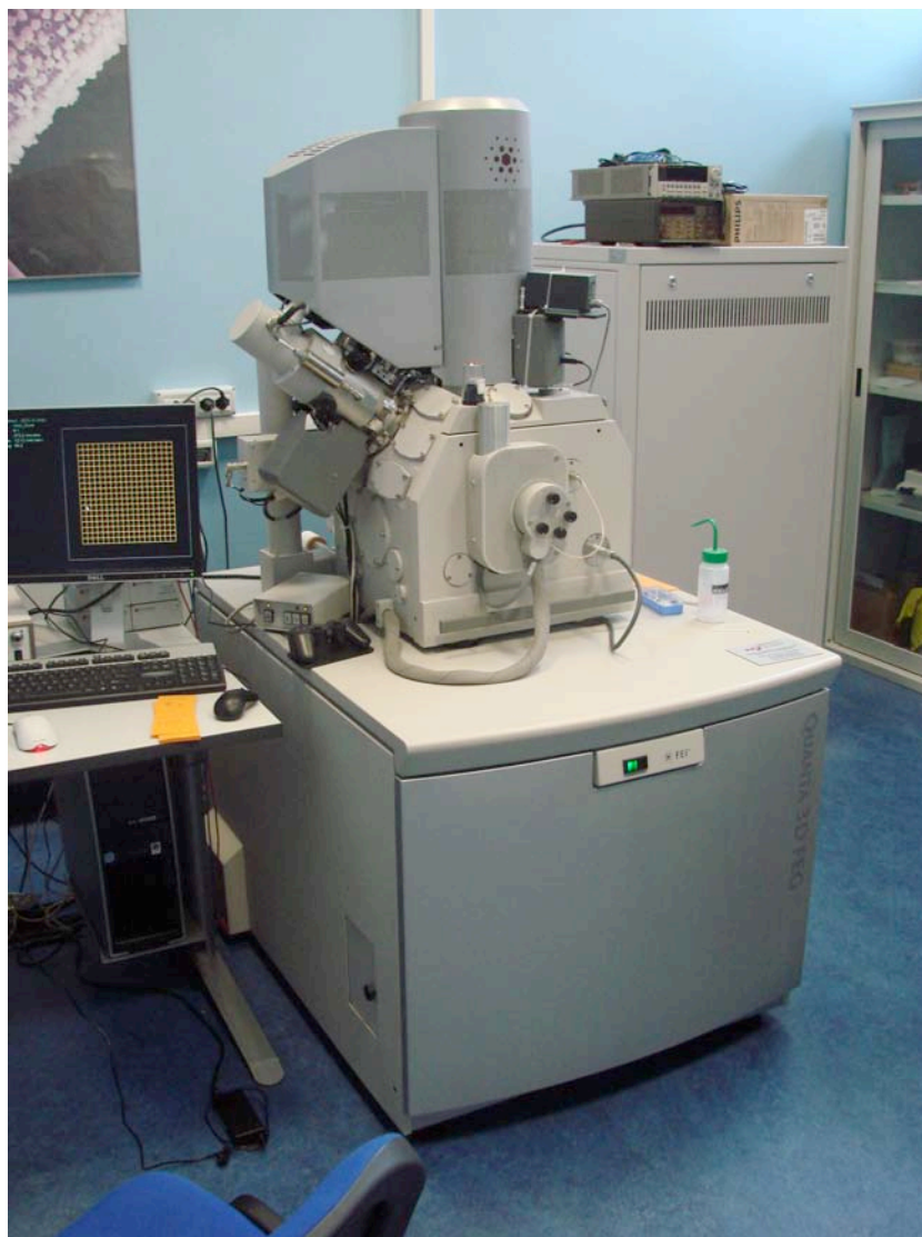
Figure C.4. Picture of the FEI Quanta 3D™ dual-beam system, at NanoFacility Piemonte ( http://www.nanofacility.it ). The electron (vertical) and the ion (52° on the left) columns collide beams in the eucentric point at a working distance of 10 mm from the electronic final lens. This powerful setup can operate under different chamber pressure from the high vacuum range up to 500 Pa of water vapor. The NPGS lithography tool control both columns via a CAD pattern and relative exposure recipe opening a wide range of applications in the nanotechnology field.
