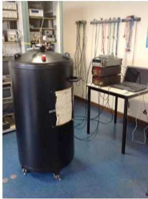
Figure A.1. The magnetically shielded Dewar for the electrical characterization of Josephson junctions, in INRIM.
