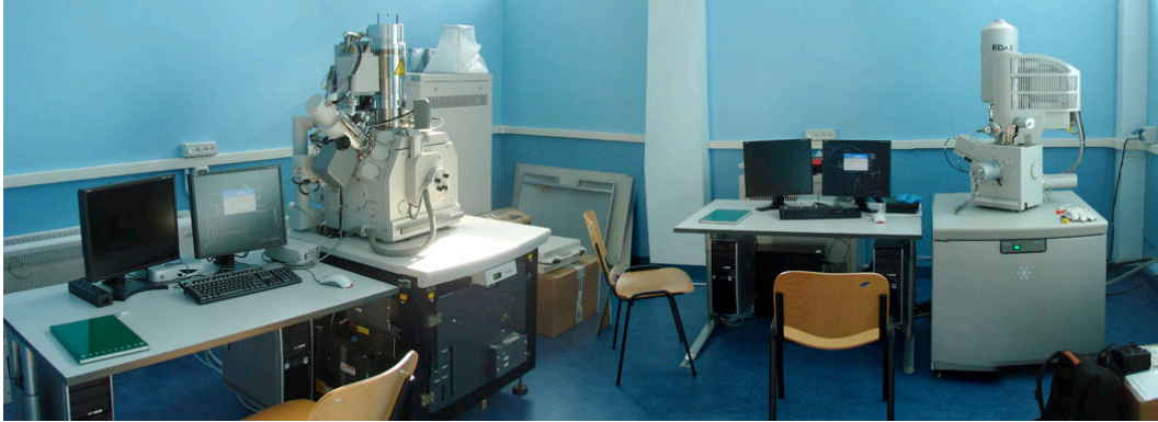
Figure 7.2. Picture of NanoFacility Piemonte Laboratory at INRIM. Left side: Quanta TM 3D FEG. Right side: Inspect F TM FEG equipped with Energy Dispersive X-ray Spectroscopy (EDS) from EDAX.
