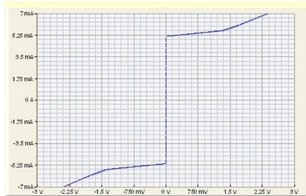
Figure 6.14. DC I - V characteristic of a 8192 junction series-connected PJVS array.
