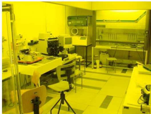
Figure C.3. Picture of the “Thin Film” ISO5 clean room Laboratory at INRIM. From left to right: two mask aligners for the optical lithography, the spinner for the resist deposition and a hood for chemical processes (substrate cleaning and resist development).
