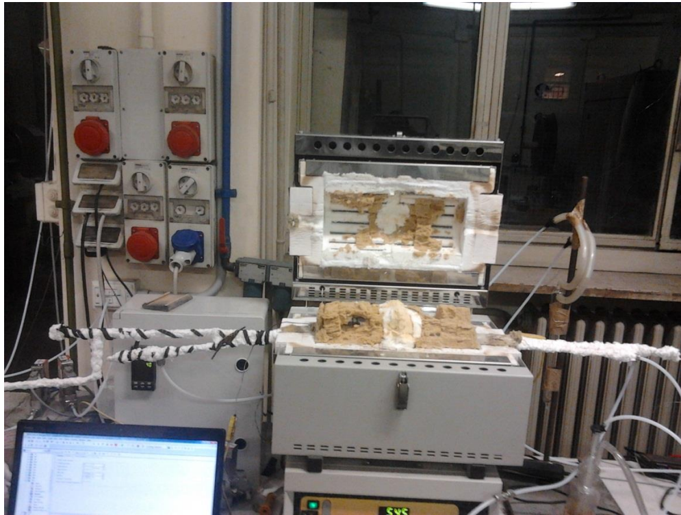
Fig.12.2 Picture of the reactor completely insulated
