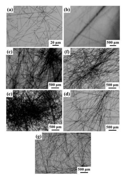
Fig. 3.1 Effect of dispersant (1 wt.%) on fibre dispersion (0.075 vol.%) in mixture of ethanol and butanol. (a) without dispersant, (b) BYK-163, (c) BYK-410, (d) BYK-2150, (e) BYK-9077, (f)BYK-9076, (g) Triton X-100.
