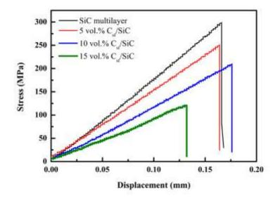
Fig. 4.1 Representative bending curve of SiC multilayer and Csf/SiC multilayer composites.
