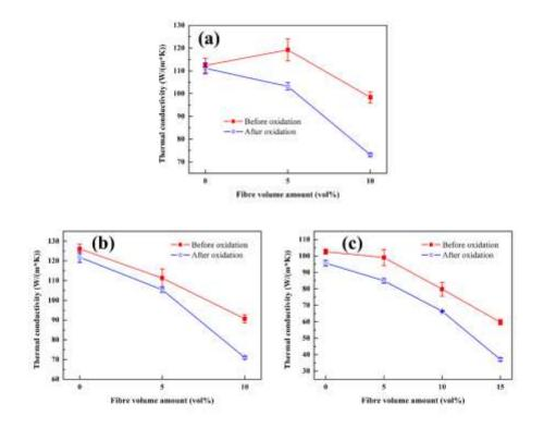
Fig. 5.13 Thermal conductivities of SiC multilayer and C<sub>st</sub>/SiC multilayer composites before and after oxidation in (a) X, (b) Y and (c) Z directions.
