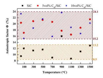
Fig. 5.15 Anisotropic factor  $\Phi$  of SiC multilayer and C<sub>st</sub>/SiC multilayer composites at different temperature.
