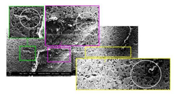
Fig. 4.3 Crack deflection in 5vol.% Cst/SiC multilayer composite.
