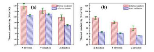
Fig. 5.14 Thermal conductivities comparison of (a) 5 and (b) 10 vol.% C<sub>st</sub>/SiC multilayer composites in X, Y and Z directions at room temperature before and after oxidation.
