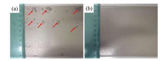
Fig. 3.5 Comparison of (a) fibre aggregation and (b) good fibre dispersion in C<sub>st</sub>/SiC green tapes.
