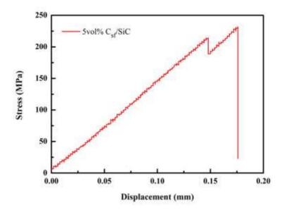
Fig. 4.2 Ladder-like bending curve in 5vol% Cst/SiC multilayer composite.
