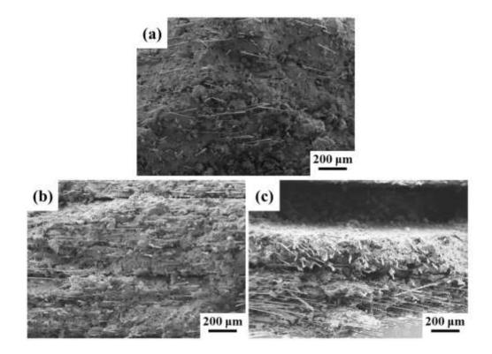
Fig. 3.8 Fracture surface of  $C_{sf}$ /SiC multilayers with different fibre amount after debinding. (a) 5 vol.%, (b) 10 vol.% and (c) 15 vol.%.
