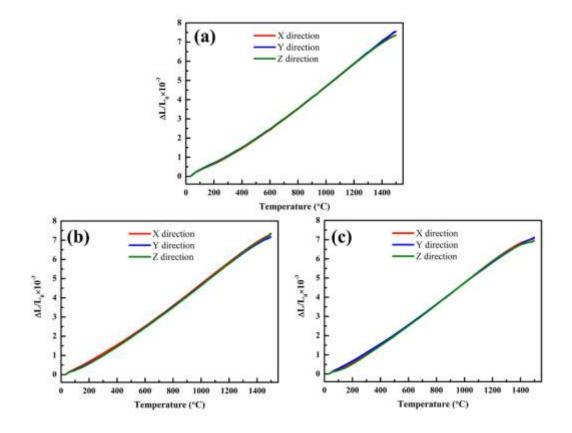
Fig. 5.3 The relative length changes of (a) SiC, (b) 5 and (c) 10 vol.% C<sub>sf</sub>/SiC multilayer composites in different directions from room temperature to 1500 °C.
