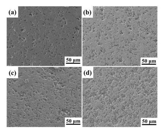
Fig. 3.9 Representative morphologies of sintered SiC multilayer and  $C_{sf}$ /SiC multilayer composites. (a) SiC multilayer, (b) 5 vol.%, (c) 10 vol.% and (d) 15 vol%  $C_{sf}$ /SiC multilayer composites.
