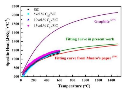
Fig. 5.2 Temperature dependence of specific heat capacity of SiC multilayer and  $C_{st}$ /SiC multilayer composites. The red line is the fitting curve in Munro's work [355], the olive line is the fitting result in present work, and purple line is the specific heat of graphite [356].
