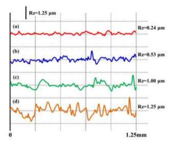
Fig. 3.6 Roughness profiles of upper-side (in contact with air) of SiC and C<sub>sf</sub>/SiC green tapes (a)
