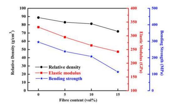
Fig. 4.4 Relationships among fibre content, relative density and elastic modulus or bending strength of SiC multilayer and  $C_{st}$ /SiC multilayer composites.
