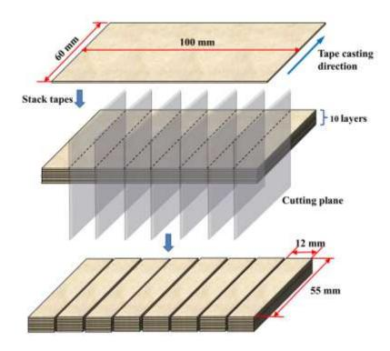
Fig. 2.4 Preparation process for green specimens for bending test.
