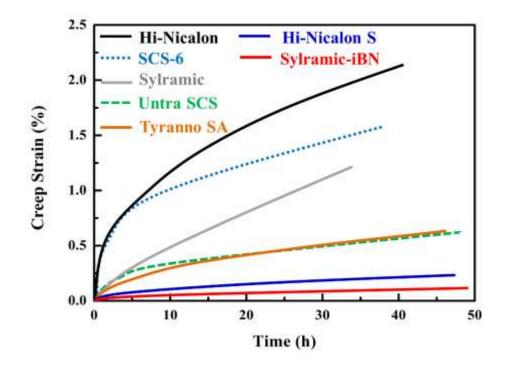
Fig. 1.2 Typical creep curves for SiC fibres tested at 1400 °C in air under a constant stress of 270 MPa [153].
