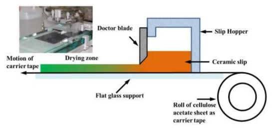
Fig. 1.11 Schematic diagram of the tape casting process [318].
