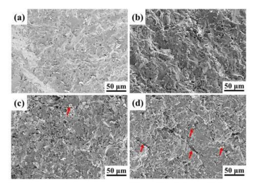
Fig. 4.7 Fracture surface of SiC multilayer and C<sub>sf</sub>/SiC multilayer composites. (a) SiC multilayer,
