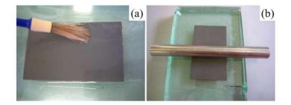
Fig. 2.2 Stacking process of green multilayer samples. (a) Paint gluing solution and (b) Removal air inclusion.
