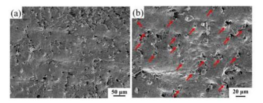
Fig. 3.7 Cross section surface of stacked green tapes of 10 vol.% C<sub>sf</sub>/SiC. (a) lower magnification and (b) higher magnification.
