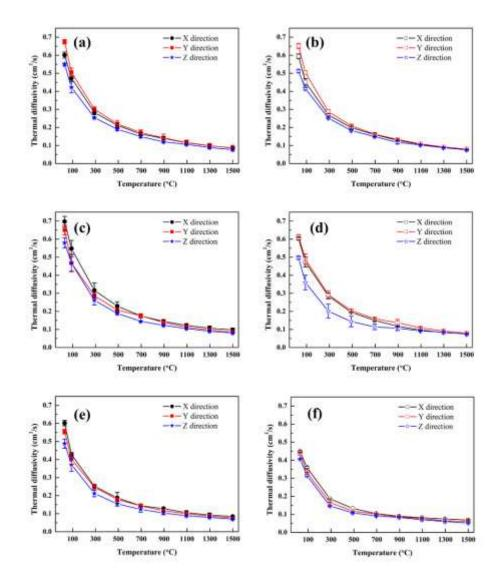
Fig. 5.6 Thermal diffusivities-temperature relationship of (a) (b) SiC multilayer, (c) (d) 5 and (e) (f) 10vol% C<sub>sf</sub>/SiC multilayer composites in three directions. (a) (c) (e) are before oxidation treatment and (b) (d) (f) are after oxidation treatment, respectively.
