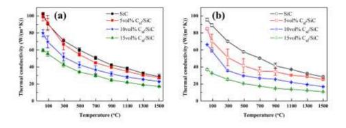
Fig. 5.9 Thermal conductivities of SiC multilayer and  $C_{sf}$ /SiC multilayer composites in Z direction from 30 to 1500 °C (a) before and (b) after oxidation treatment.
