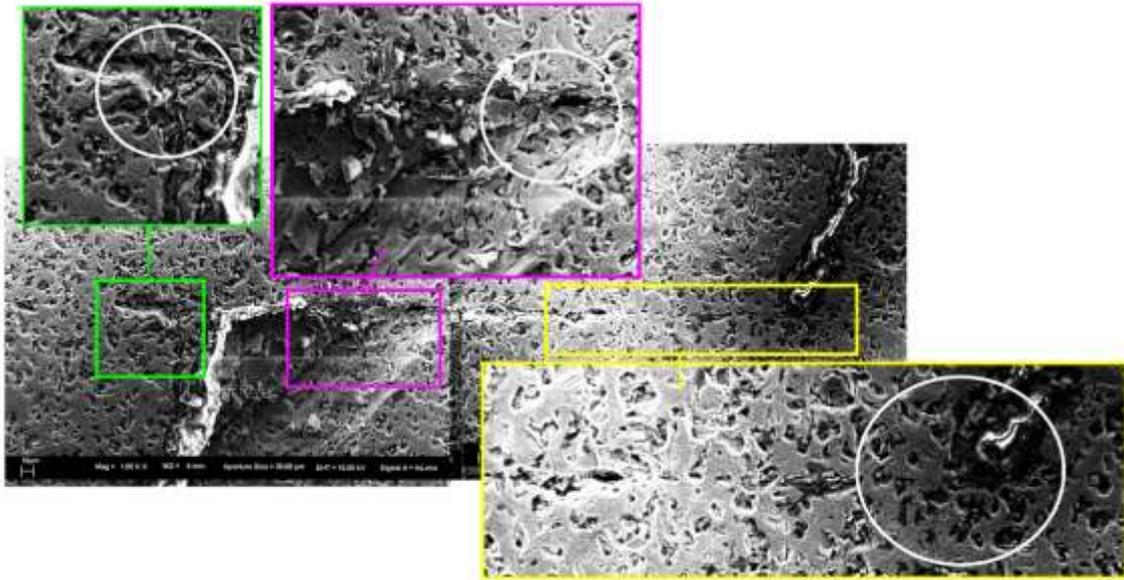
Fig. 4.3 Crack deflection in 5vol.% C<sub>sf</sub>/SiC multilayer composite.
