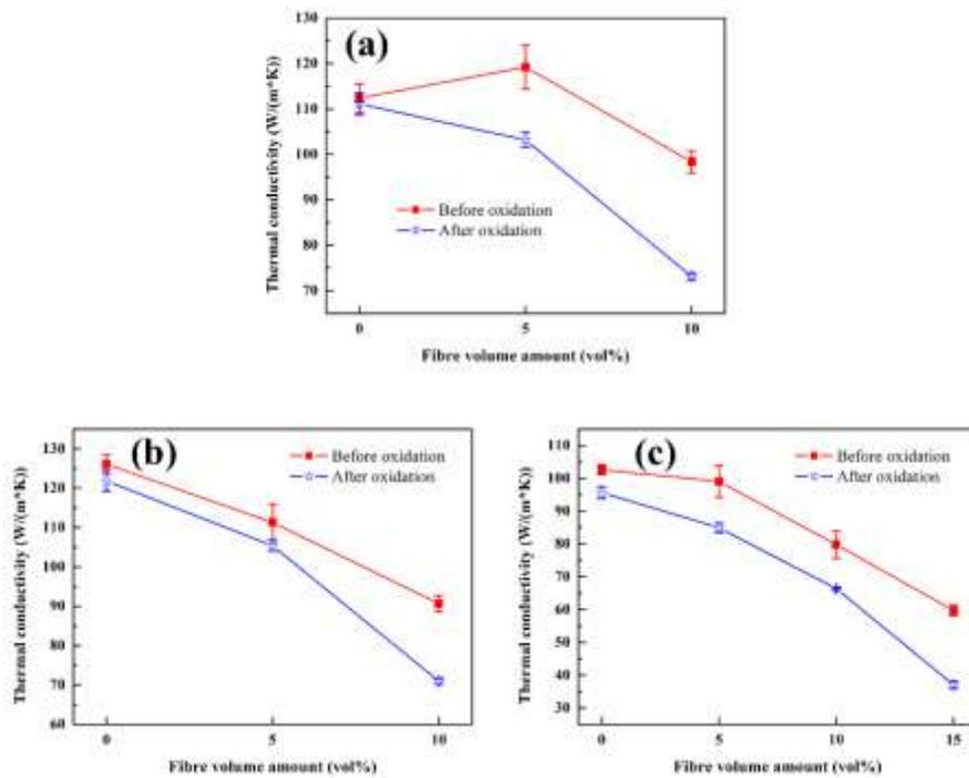
Fig. 5.13 Thermal conductivities of SiC multilayer and C<sub>sf</sub>/SiC multilayer composites before and after oxidation in (a) X, (b) Y and (c) Z directions.
