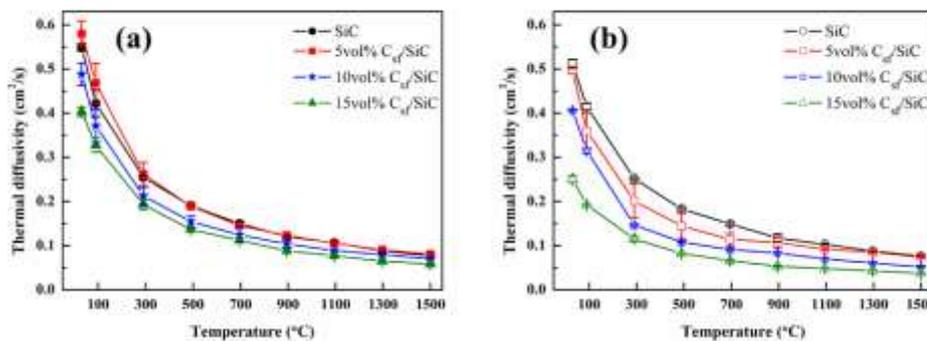
Fig. 5.7 Thermal diffusivities of SiC multilayer and C<sub>sf</sub>/SiC multilayer composites in Z direction from 30 to 1500 °C (a) before and (b) after oxidation treatment.
