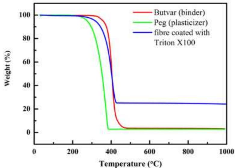
Fig. 2.9 Decomposition curves of binder, plasticizer and fibre dispersant.
