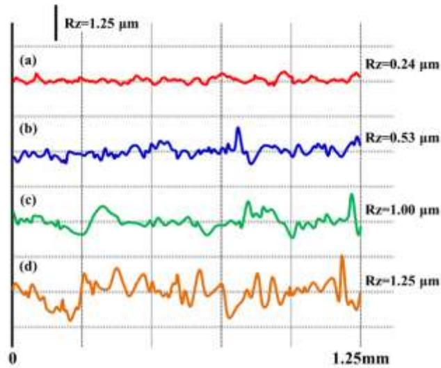
Fig. 3.6 Roughness profiles of upper-side (in contact with air) of SiC and  $C_{sf}/SiC$  green tapes (a) SiC, (b) 5 vol.%, (c) 10 vol.%, (d) 15 vol.%  $C_{sf}/SiC$  green tapes.
