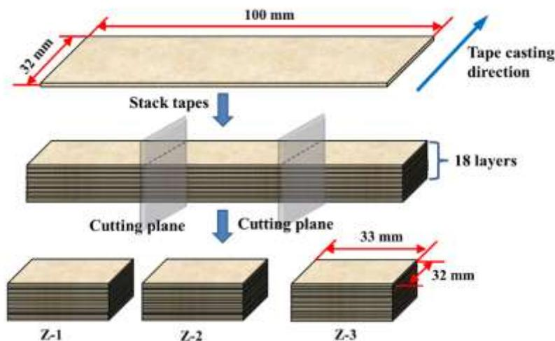
Fig. 2.6 Preparation process of green samples for thermal properties test in Z direction.
