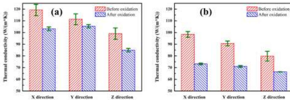
Fig. 5.14 Thermal conductivities comparison of (a) 5 and (b) 10 vol.% C<sub>sf</sub>/SiC multilayer composites in X, Y and Z directions at room temperature before and after oxidation.
