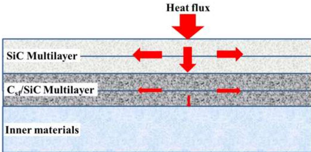
Fig. 5.16 Prospective application of C<sub>sf</sub>/SiC multilayer for thermal protection system.
