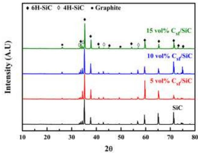
**Fig. 3.10** XRD patterns of SiC multilayer and C<sub>sf</sub>/SiC multilayer composites.
