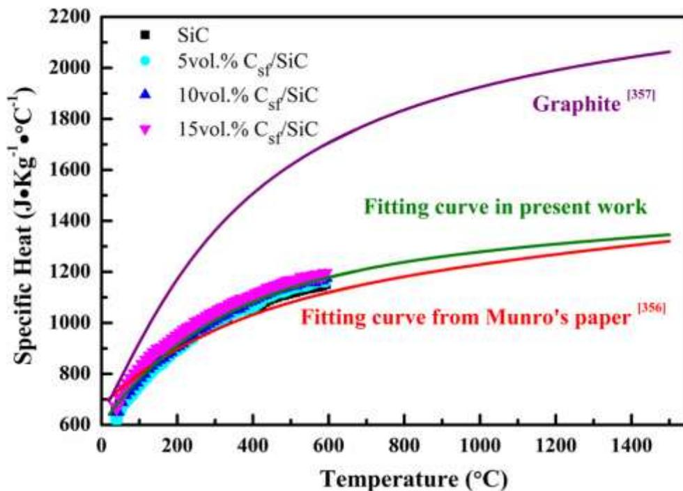
Fig. 5.2 Temperature dependence of specific heat capacity of SiC multilayer and C<sub>sf</sub>/SiC multilayer composites. The red line is the fitting curve in Munro's work [355], the olive line is the fitting result in present work, and purple line is the specific heat of graphite [356].
