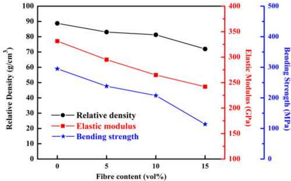
Fig. 4.4 Relationships among fibre content, relative density and elastic modulus or bending strength of SiC multilayer and C<sub>sf</sub>/SiC multilayer composites.
