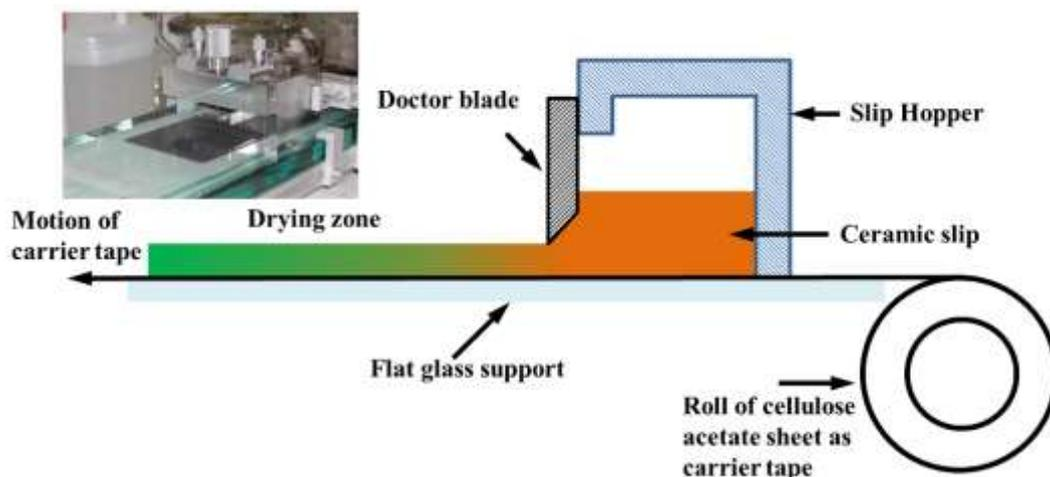
Fig. 1.11 Schematic diagram of the tape casting process [318].
