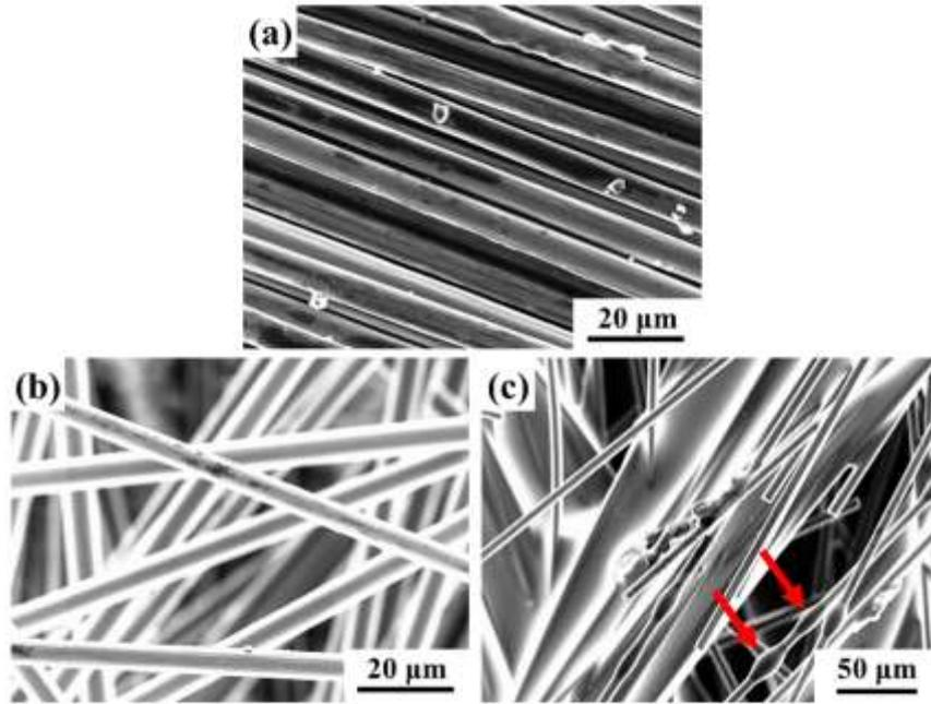
**Fig. 3.3** Microstructure of (a) original commercial fibres, (b) dried fibres dispersed in solvent without any dispersant, (c) dried fibres dispersed in solvent with Triton X100.
