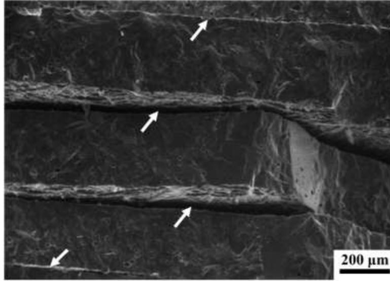
Fig. 5.12 Fracture surface of sintered SiC multilayer buckle [262].
