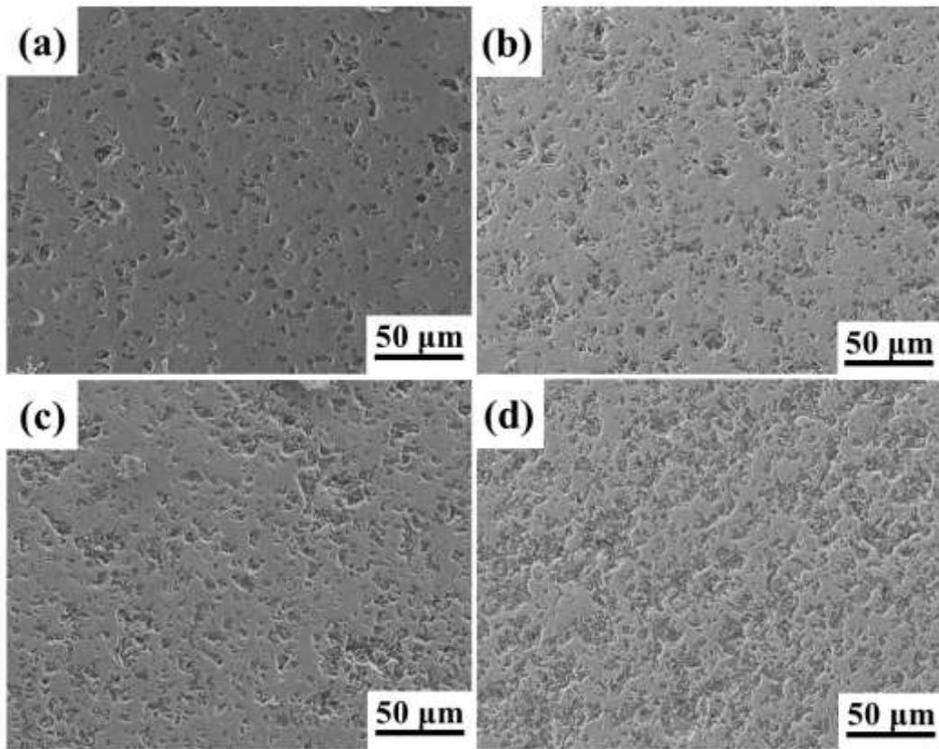
**Fig. 3.9** Representative morphologies of sintered SiC multilayer and C<sub>sf</sub>/SiC multilayer composites. (a) SiC multilayer, (b) 5 vol.%, (c) 10 vol.% and (d) 15 vol% C<sub>sf</sub>/SiC multilayer composites.
