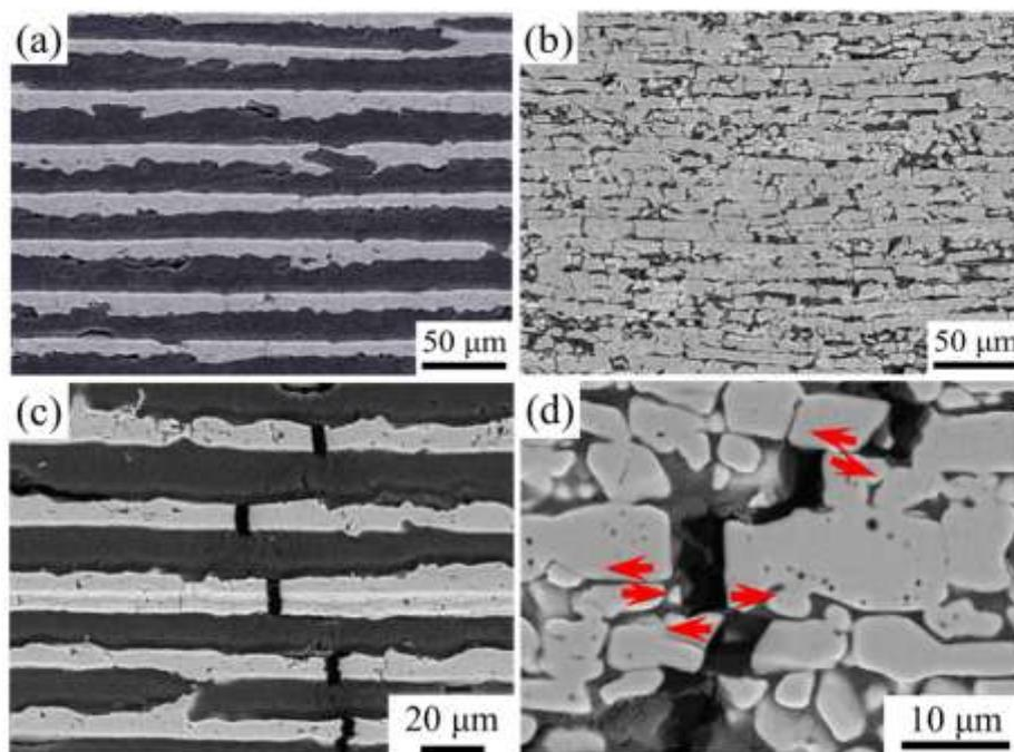
Fig. 1.9 Typical microstructure and fracture behavior of  $\text{Al}_2\text{O}_3/\text{PMMA}$  composites prepared by Munch et al. [299]. (a) Microstructure of lamellar architecture, (b) Microstructure of brick-and-mortar architecture, (c) Fracture behavior of lamellar architecture and (d) Fracture behavior of brick-and-mortar architecture.
