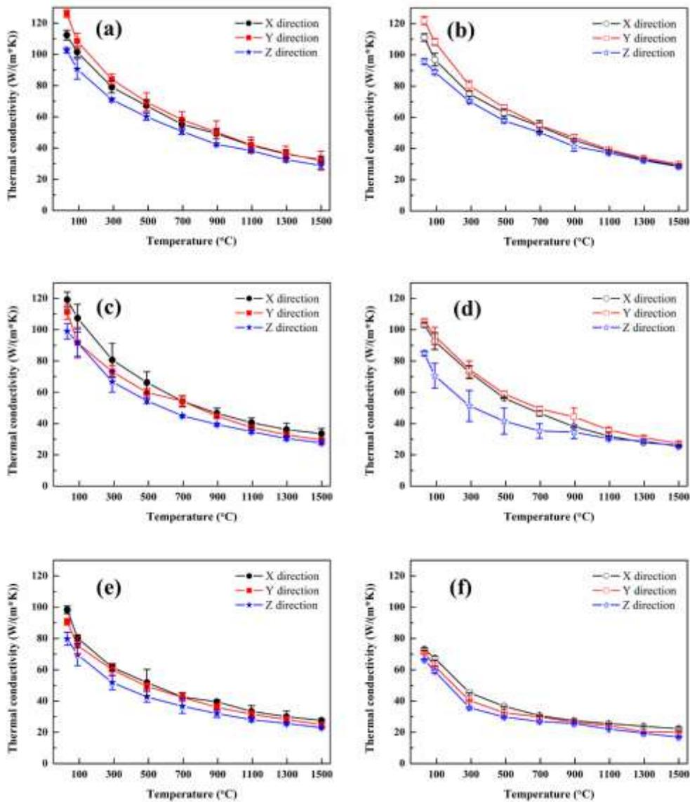
Fig. 5.8 Thermal conductivities-temperature relationship of (a) (b) SiC multilayer, (c) (d) 5 and (e) (f) 10vol% C<sub>sf</sub>/SiC multilayer composites in three directions. (a) (c) (e) are before oxidation treatment and (b) (d) (f) are after oxidation treatment, respectively.
