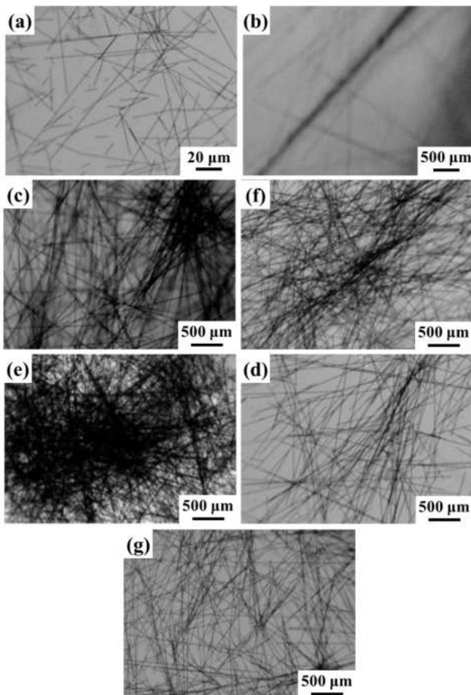
**Fig. 3.1** Effect of dispersant (1 wt.%) on fibre dispersion (0.075 vol.%) in mixture of ethanol and butanol. (a) without dispersant, (b) BYK-163, (c) BYK-410, (d) BYK-2150, (e) BYK-9077, (f)BYK-9076, (g) Triton X-100.
