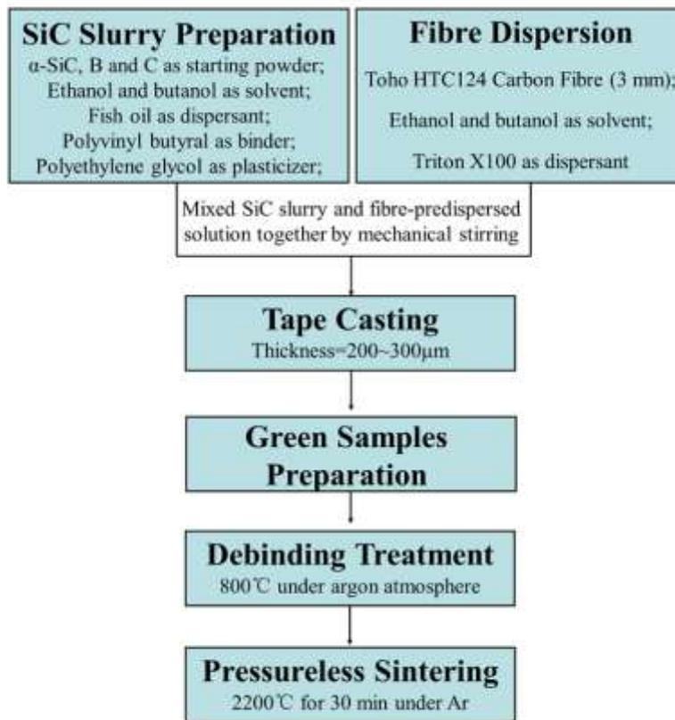
Fig. 2.1 Preparation process of C<sub>sf</sub>/SiC multilayer composite by tape casting and pressureless sintering.
