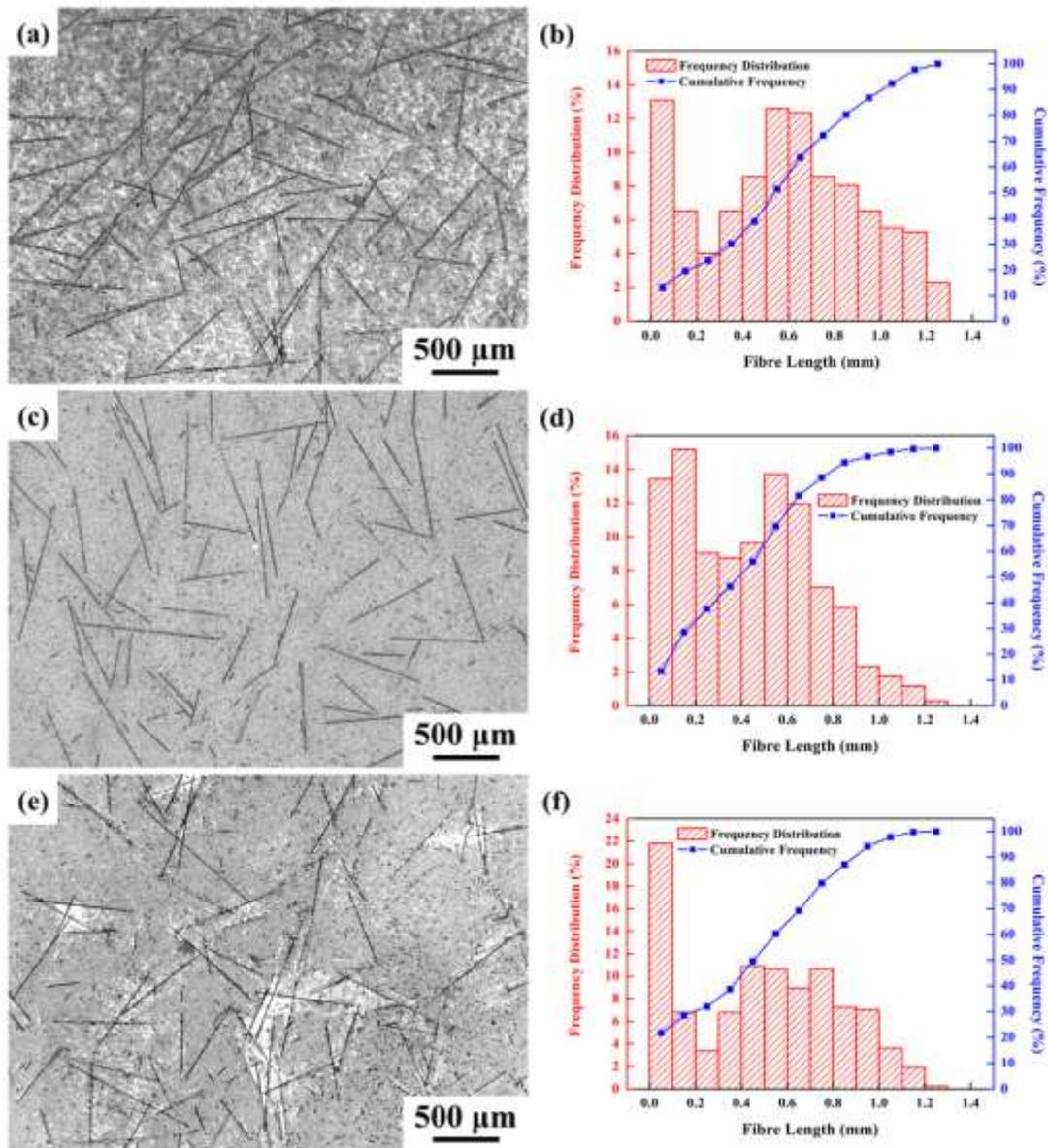
**Fig. 3.4** Typical fibre length distribution and statistical results after mechanical mixing of SiC slurry and fibre-predispersed solution. (a), (c) and (e) are the typical length distribution in the slurry whose fibre amount in final sintered samples were 5, 10 and 15 vol.% respectively. (b), (d) and (f) are the corresponding statistical results of (a), (c) and (e), respectively.
