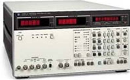
Figure 5.7: HP Impedance Analyzer for C-V measurement
