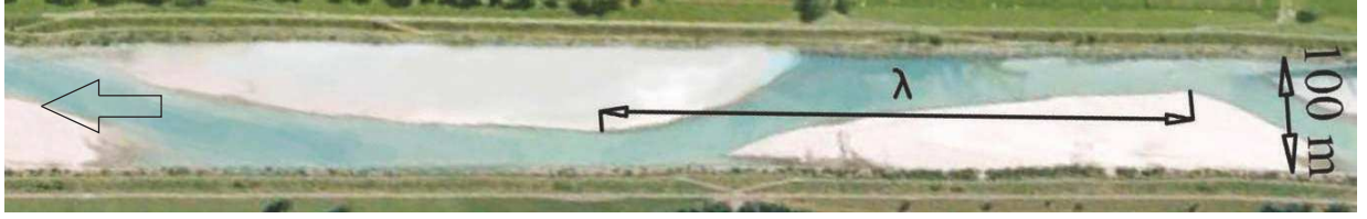
Fig. 1: Picture of an alternate bar pattern in the Rhine River, near Vaduz, Liechtenstein (47°06′40″N, 9°31′02″E). The bar wavelength, \lambda , is shown; the arrow indicates the flow direction.
