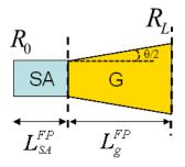
Figure 3.4: Schematic of a QD ML laser with tapered gain section (G) and reverse biased saturable absorber (SA).
