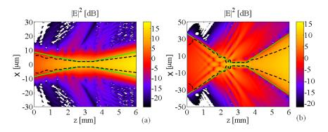
Figure 3.5: BPM simulation of the field profile evolution during forward and backward propagation across the tapered device with  $\theta = 0.3^{\circ}$  (a) and  $\theta = 1.5^{\circ}$  (b). Black dashed lines represent a reduction of -3 dB with respect to the maximum field intensity in each longitudinal section of the device. Continuous green lines represent the waveguide profile,  $x = \pm W(z)/2$ , being W(z) the ridge width as a function of the longitudinal coordinate z.
