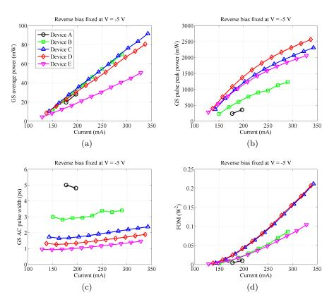
Figure 3.11: Average power (a), peak power (b), deconvoluted autocorrelation (AC) pulse width (c) and FOM (d) at the fixed reverse-bias voltage V = -5 V and as a function of the injection current for devices A (square), B (circle), C (upward-pointing triangle), D (diamond) and E (downward-pointing triangle) in Fig. 3.10.
