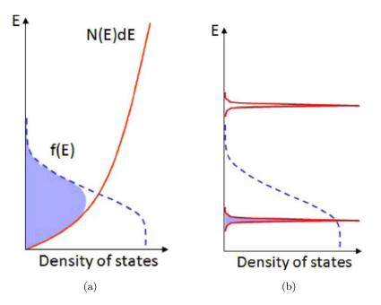
Figure 1.1: (a) Density of states, Fermi function and density of carriers for a bulk semiconductor. (b) Dirac delta function density of states for QD material (from reference [6]).
