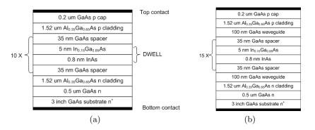
Figure 1.6: Schematics diagram of the epitaxial structure for InAs/InGaAs QDbased device with active region consisting of 10 stacks (a) and 15 stacks (b) of QD layers respectively.
