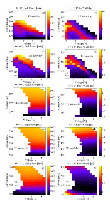
Figure 3.7: Maps of pulse peak power and pulse width as a function of the current applied to the gain section and voltage applied to the SA for devices with  $\theta = 0^{\circ}$ ,  $0.3^{\circ}$ ,  $0.6^{\circ}$ ,  $1^{\circ}$  and  $1.5^{\circ}$ .
