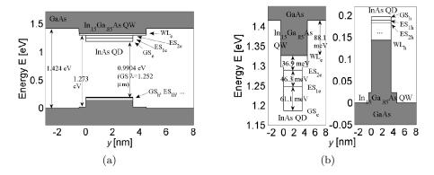
Figure 1.8: Schematic of the energy band structure of a realistic  $InAs/In_{0.15}Ga_{0.85}As$  DWELL layer. The interband (a) and intraband (b) transition characteristic energies are reported. The wetting layer band edge, representing the transition from confined QD states to a continuum of 2D delocalized states, is highlighted (from reference [24]).
