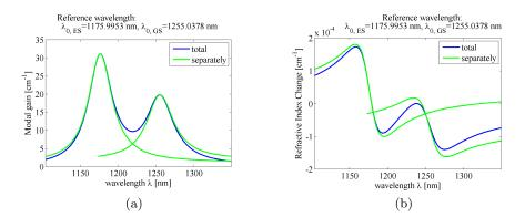
Figure 2.3: Simple schematic of the gain (a) and refractive index change (b) spectrum. The blue curves represent the total spectrum profile, while the green curves represent the profiles of these two parameters when we consider two distinct bands.
