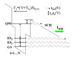
Figure 2.2: Schematic of the energy diagram in a reverse bias condition. Symbol  $\rightsquigarrow$  denotes tunneling processes. Double arrows  $\updownarrow$  indicate possible capture (relaxation) and escape processes.
