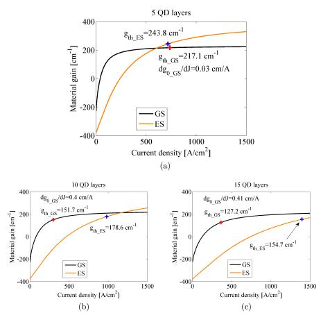
Figure 3.8: Dependence of GS (black) and ES (orange) material gain on the injection current density for devices with active region consisting of 5 (a), 10 (b), 15 (c) QD layers. Corresponding threshold gains (plus marker) and differential gains at GS/ES transitions are also indicated.
