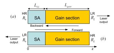
Figure 3.12: Schematic of the two-section ML laser with output from the gain section side facet (a) and the configuration with output from the SA side facet (b).
