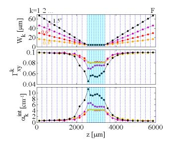
Figure 3.6: Ridge width  $W_k$ , field confinement factor  $\Gamma_{xy,k}$  and internal losses  $\alpha_{int,k}$  for tapered devices with  $\theta = 0.3^{\circ}, 0.6^{\circ}, 1^{\circ}, 1.5^{\circ}$ .
