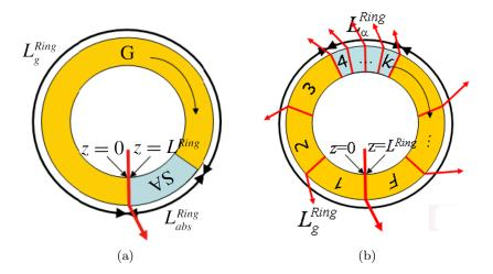
Figure 2.5: Simple schematic of the equivalent unidirectional ring laser described by the standard DDE model (a) and the MS-DDE model (b). Forward biased gain section (yellow) and the reverse biased saturable absorber (light blue) are highlighted. The simulated device consists of F isolated sections; red lines/arrows indicate the non-saturable losses introduced at each interface between adjacent sections (from reference [58]).
