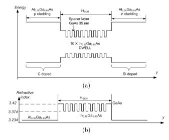
Figure 1.7: Schematics of the transversal direction variation of the energy gap (a) and the refractive index (b) for device in Fig. 1.6a.
