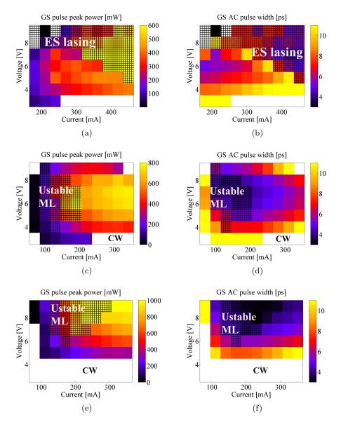
Figure 3.9: Maps of the pulse peak power and the pulse width with the same variation span of the injection current and the reverse bias voltage for 2 mm device with 5, 10, 15 QD layers. Shaded regions represent unstable ML performances, which is mainly induced by ES lasing for 5 QDL device, whereas by unbalanced gain and absorption dynamics for 10 and 15 QDL devices.
