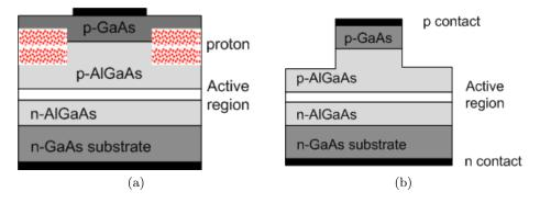
Figure 1.9: Cross-section view of the lateral confinement structures: (a) the protonimplant waveguide; (b) the ridge waveguide.
