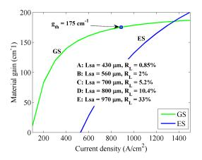
Figure 3.10: QD material gain from GS (green) and ES (blue) transitions as a function of the injection current density. The square marker represents the fixed threshold gain for the devices considered in the simulations. The corresponding SA length and the output power reflectivity are also shown.
