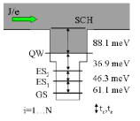
Figure 2.1: Schematic of the cascade transitions of electrons between different states in the conduction band of the QD material. Arrows indicate the capture/relaxation and escape processes of electrons.
