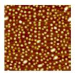
Figure 1.3:  $500 \times 500 \ nm^2$  AFM image of self-assembled InAs QDs grown on the (100) oriented GaAs substrate (from reference [18]).
