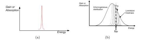
Figure 1.4: Schematics of the spectral gain profile for (a) single quantum dot and (b) an ensemble of self-assembled QDs grown by SK process.
