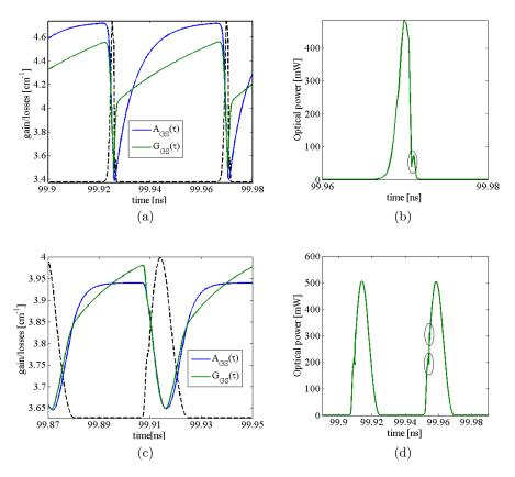
Figure 3.2: (a) Net gain profile of a ML pulse with tailing edge instability and (b) the corresponding pulse envelope; (c) Net gain profile of a ML pulse with leading edge instability and (d) the corresponding pulse envelope.
