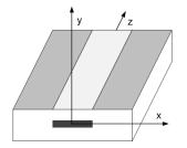
Figure 1.5: Simple schematic of edge-emitting lasers and the selected coordinate system of this thesis.
