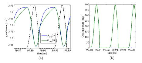
Figure 3.1: (a) Net gain profile of a stable ML pulse and (b) the corresponding pulse envelope.
