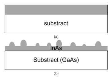
Figure 1.2: Cross-section view of (a) traditional uniform epitaxial layer growth and (b) self-assembled QDs growth based on SK process.
