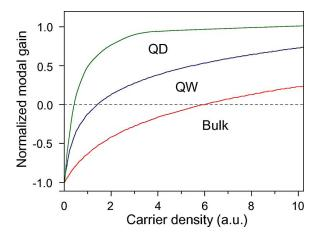
Figure 3.3: Simple schematic of the normalised modal gain as a function of the carrier density for the bulk, QW and QD materials. Figure from [11].
