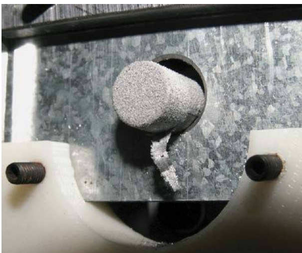
Figure 9 Evidence of delamination wear at the earliest stages of the wearing test of the Alumide specimen
